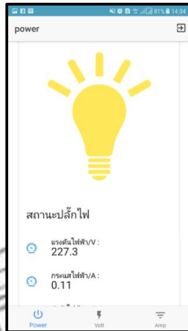
Figure 7 Figure's Application controlled on / off power.
